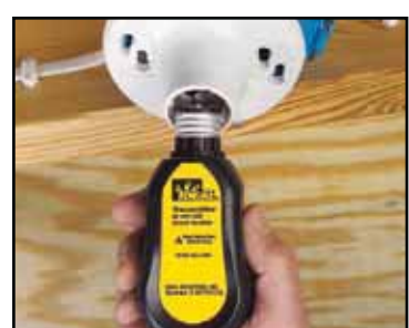
Lighting adapter allows connection to light fixtures.
