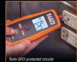
Tests GFCI protected circuits
