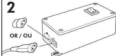
Connect flexible wire connector or link connector (large end) to the box.
