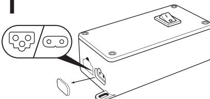
Remove 2-wire or 3-wire connector cover from box.
