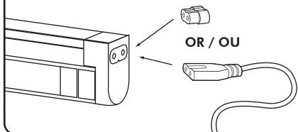
Connect the other side of the flexible wire connector or link connector to the Fluoro Bar light fixture.
