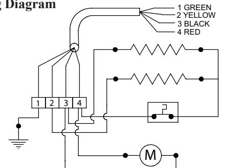
Two wattage configurations are possible: (750W or 1500W).
