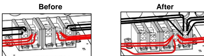
Figure 4 : Conversion from two to one supply wires
