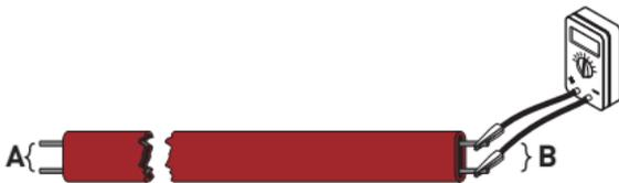
**Measure the bus-to-bus heating cable resistance** from the front end (measurement A) and the back end (measurement B) of the suspect section.
