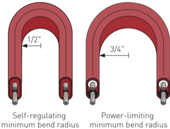
When positioning the heating cable on the pipe, do not bend tighter than 1/2" for self-regulating cables and 3/4" for power-limiting cables.
