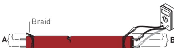
The approximate location of the fault, expressed as a percentage of the heating cable length from the front end (A), is:
