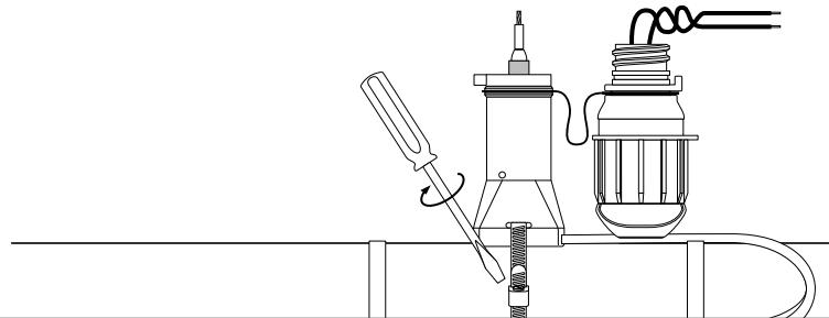
**Note:** For 1-in (25-mm) and smaller pipes use adapter (purchased separately) between stand and pipe.
